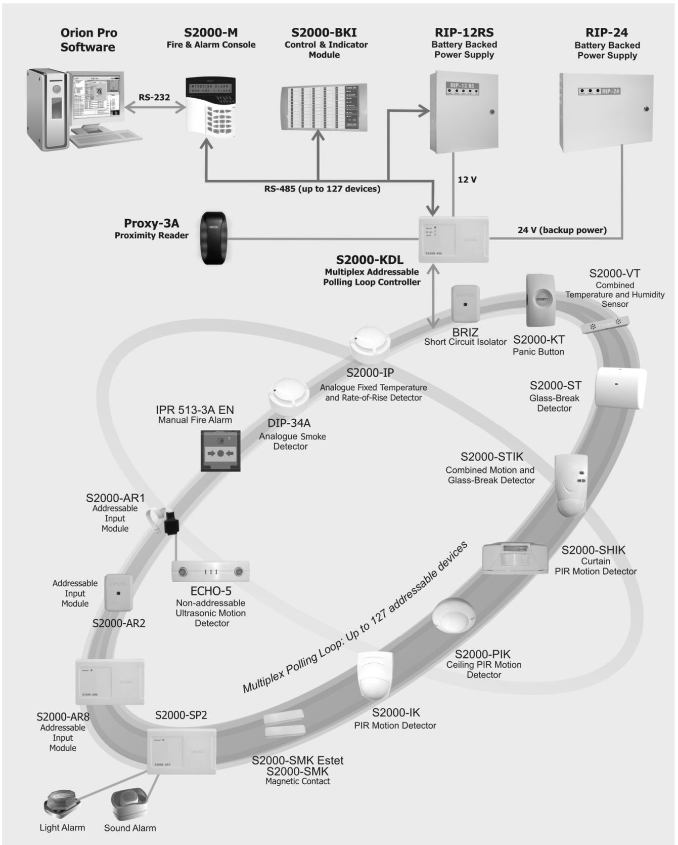
Figure 1. Analogue Addressable Message Transferring Systems Based on S2000-KDL
