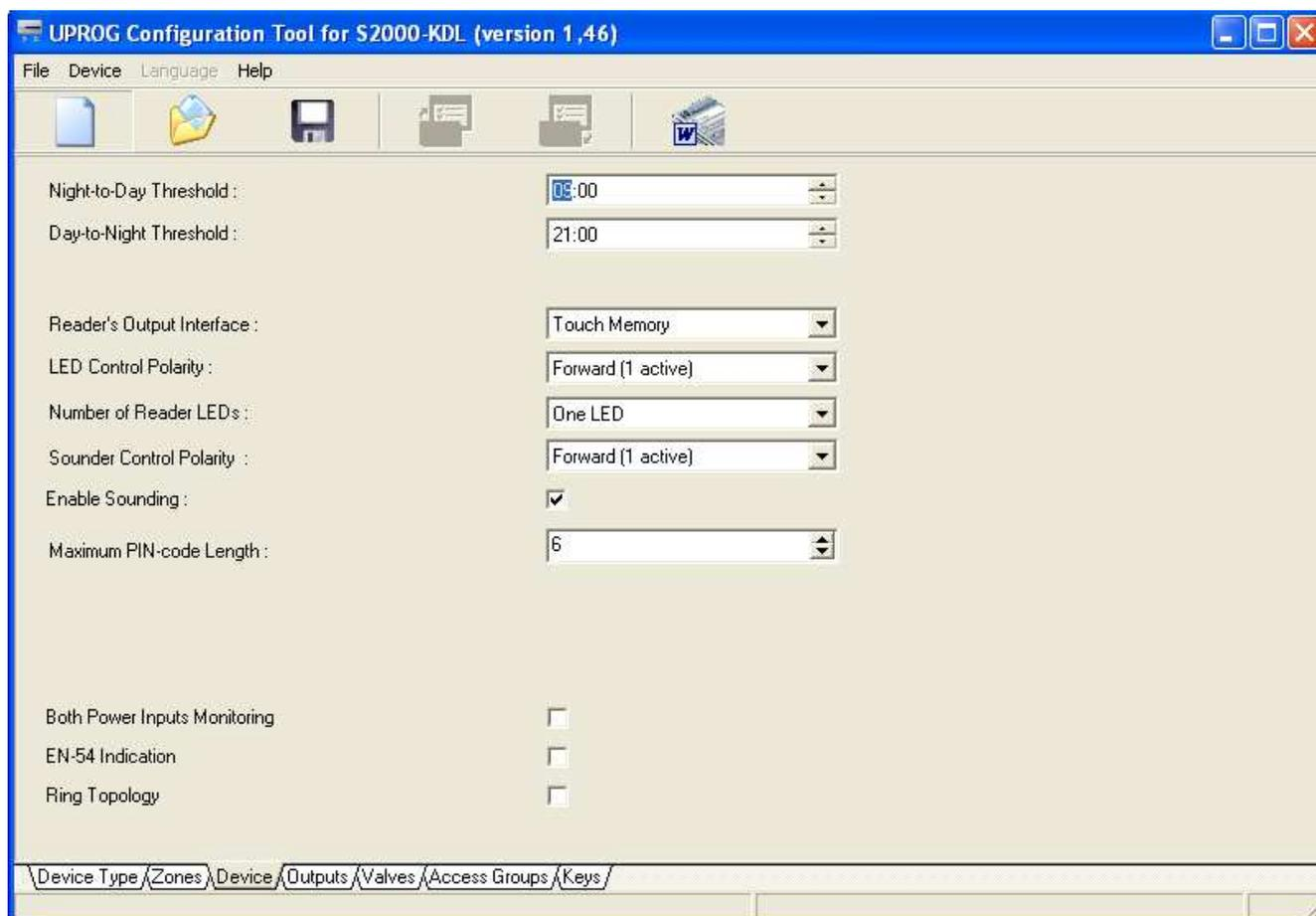
**Figure 13. Settings of the S2000-KDL and the External Reader**
