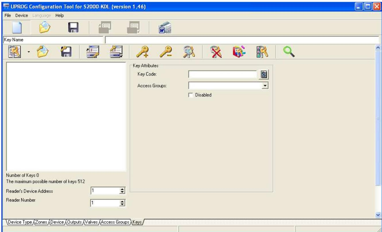
**Figure 18. Programming electronic keys in the UProg**
