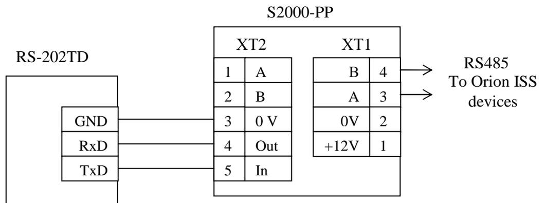
**Figure 12. Connecting the Transmitter to the S2000-PP**
