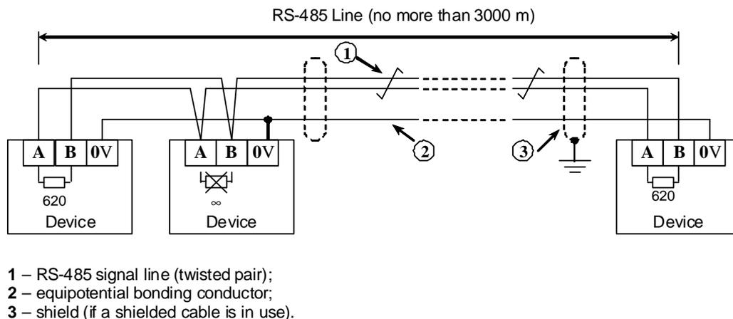
Figure 13. The Schematic for Connecting Devices to the RS-485 Interface
