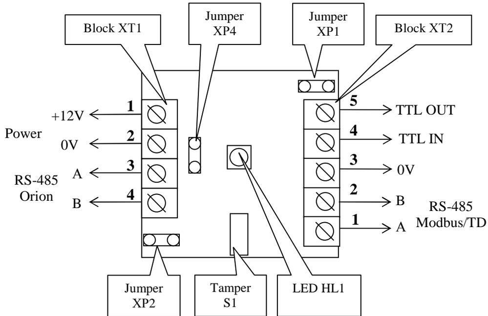
**Figure 3. S2000-PP Printed Circuit Board**
