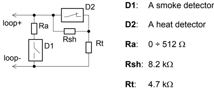
**Figure 5. Smoke and Heat Detectors into a Fire Loop of the Type 2 Connecting Diagram**
