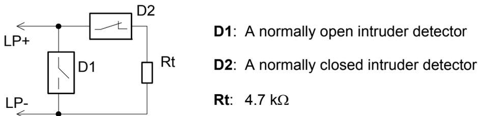
**Figure 7. Wiring Intrusion Detectors into Alarm Loops of the Type 4**
