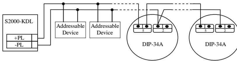
Figure 1. Connection Diagram
