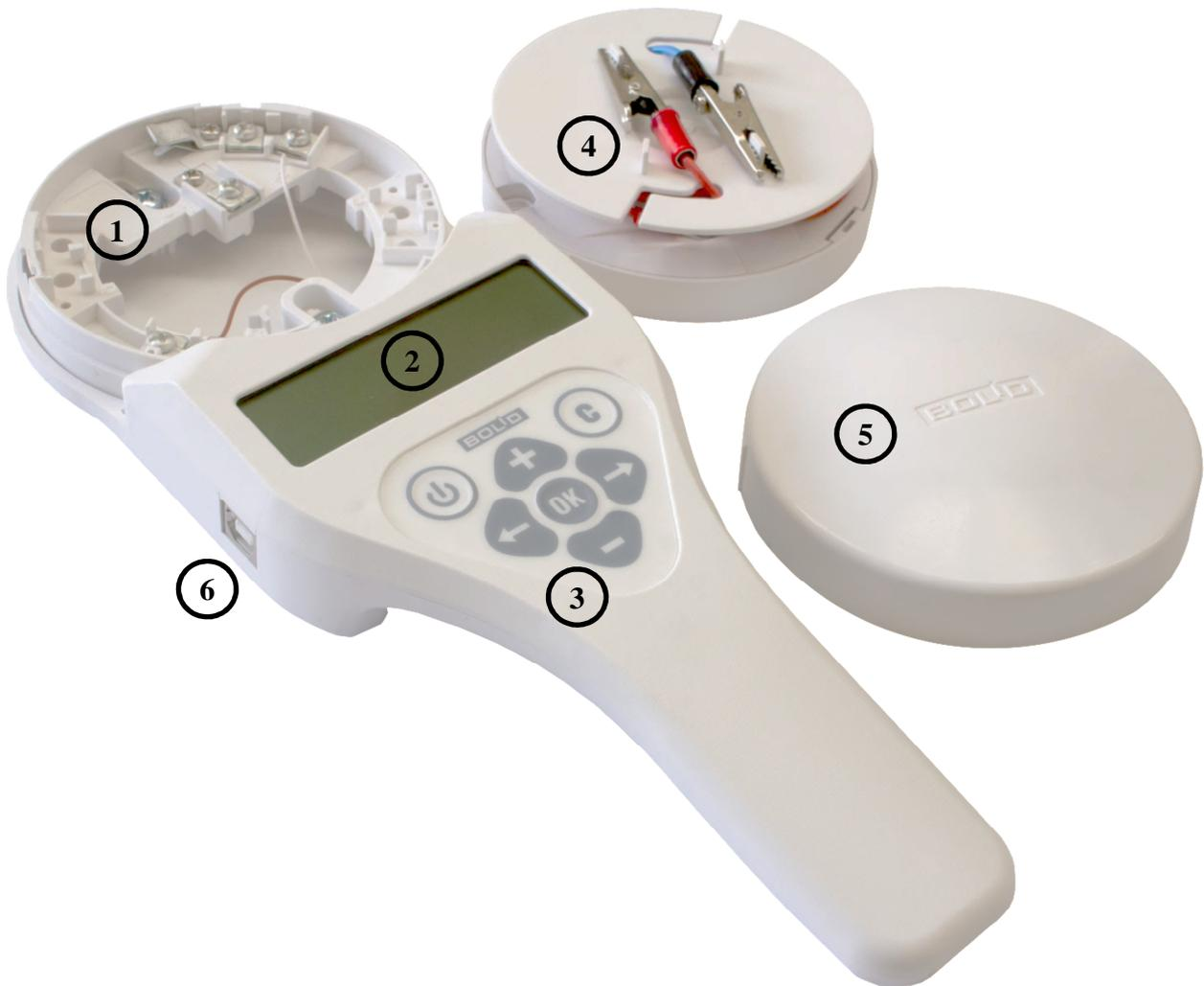
**Figure 1. Appearance and Controls of the Programmer**
