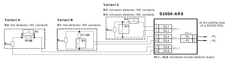
The above diagram shows wiring the S2000-AR8 to the polling loop of an S2000-KDL / S2000-KDL-2I as well as standard variants for wiring non-addressable detectors to the S2000-AR8 monitored circuit (detector loop) contacts DL1 to DL8.
