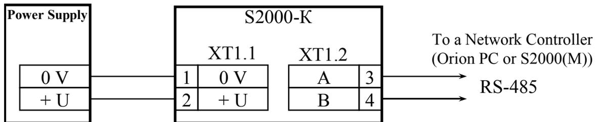
Figure 2. S2000-K Wiring Diagram
