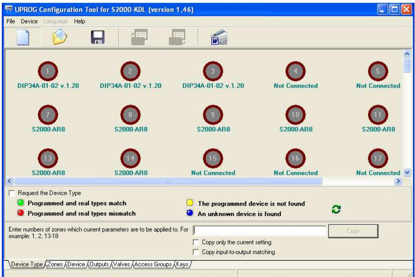
Figure 12. UProg Window for Configuring the S2000-KDL
