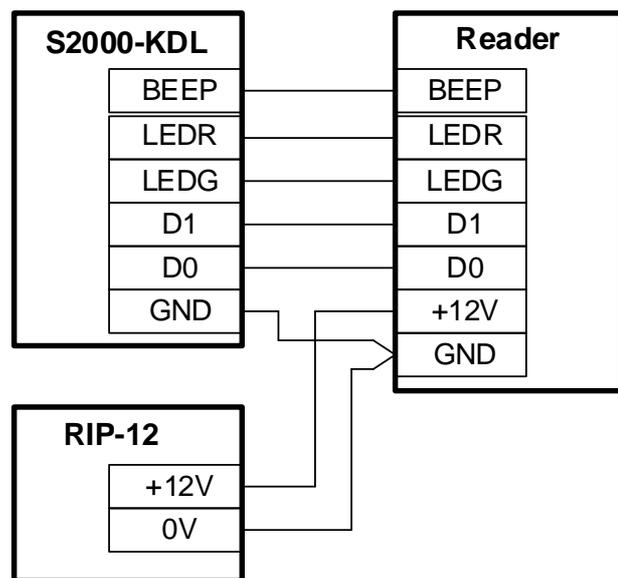
**Figure 10. Connecting Readers with Wiegand Output Interface to the S2000-KDL**
