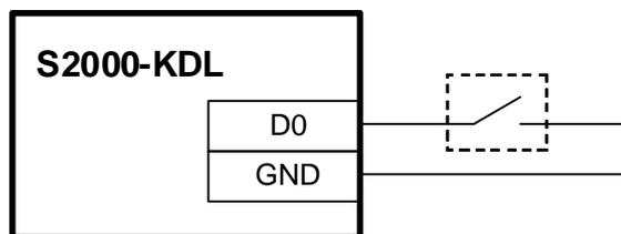
**Figure 11. Wiring the Arming Request Button**
