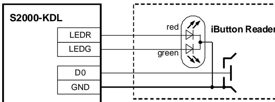
**Figure 8. Connecting a Dallas iButton Reader to the S2000-KDL**
