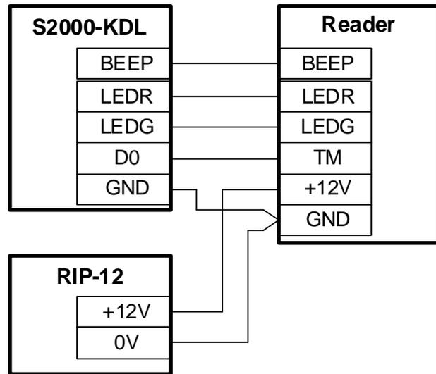
**Figure 9. Connecting Readers with Touch Memory Output Interface to the S2000-KDL**
