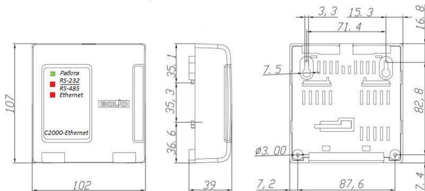
Figure 8. Overall and Mounting Dimensions
