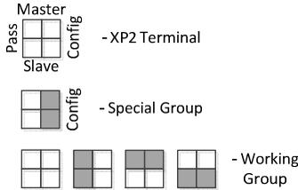
**Figure 1. Selecting a Group of S2000-Ethernet Operation Modes**
