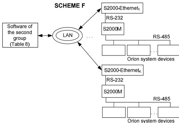
**Figure 3. Common Diagrams for Using the S2000-Ethernet as a Component of an Orion System**
