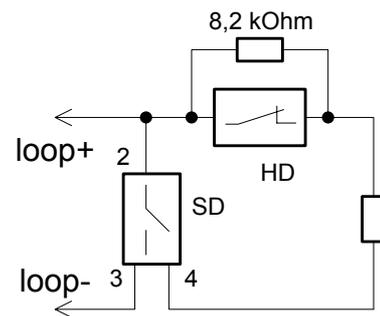
**Scheme of heat detector connection, loop type 3**
