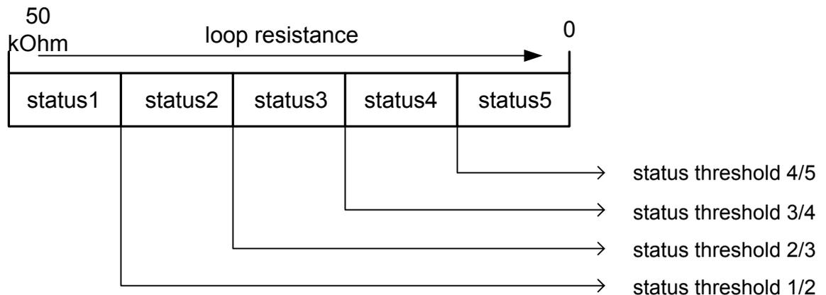
**Figure 1. Statuses and status thresholds of programmable auxiliary loop**
