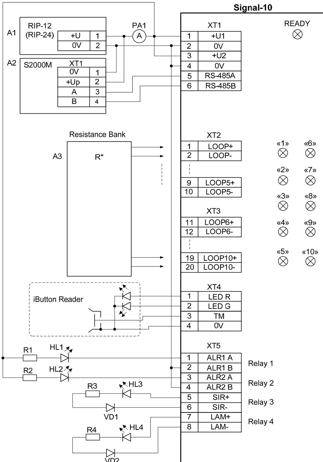
**Figure 17. Wiring the Signal-10 for Operability Inspection**
