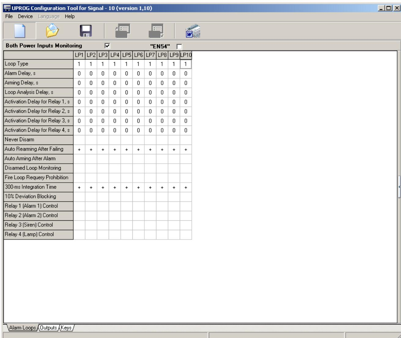
Figure 11. UProg Work Window for Configuring the Signal-10
