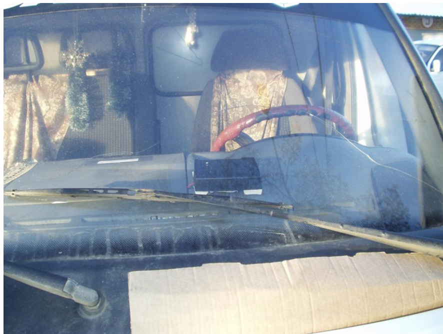
Figure 2. An Example of Attaching the Tracker above the Dashboard
