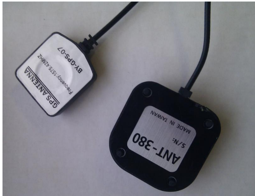
Figure 4. Appearance of GPS Antennas
