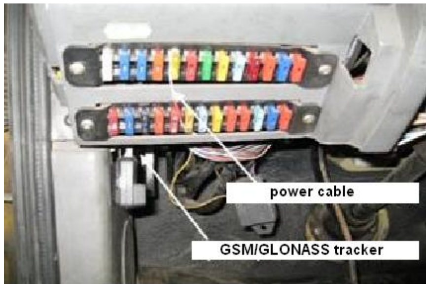
Figure 3. An Example of Attaching the Tracker under the Dashboard (Secured Mounting)
