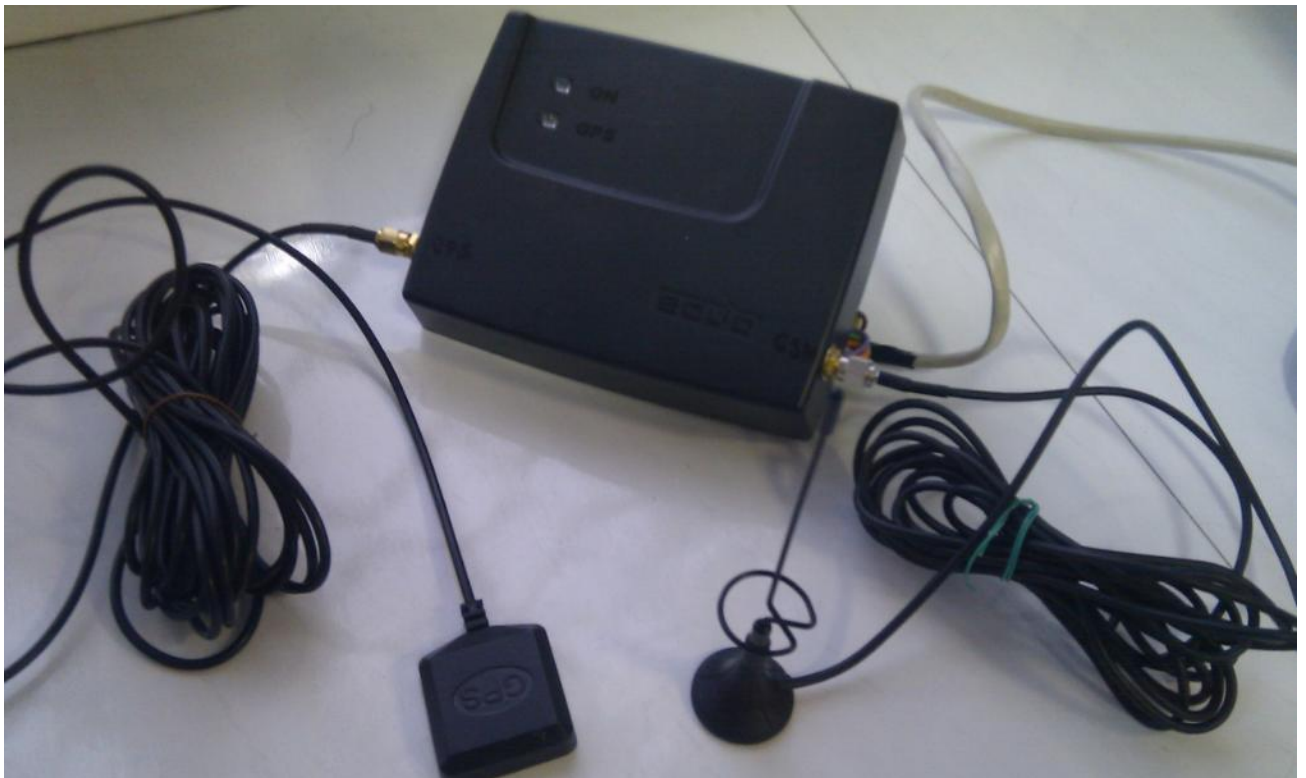
Figure 5. Appearance of the UR-03 rev.01 Tracker with GPS Antenna and GSM Antenna
