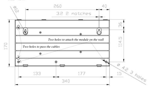
Figure 1. View and Overall and Mounting Dimensions of the Potok-BKI Module
