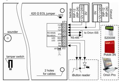
Figure 3. Module's Connection Diagram
