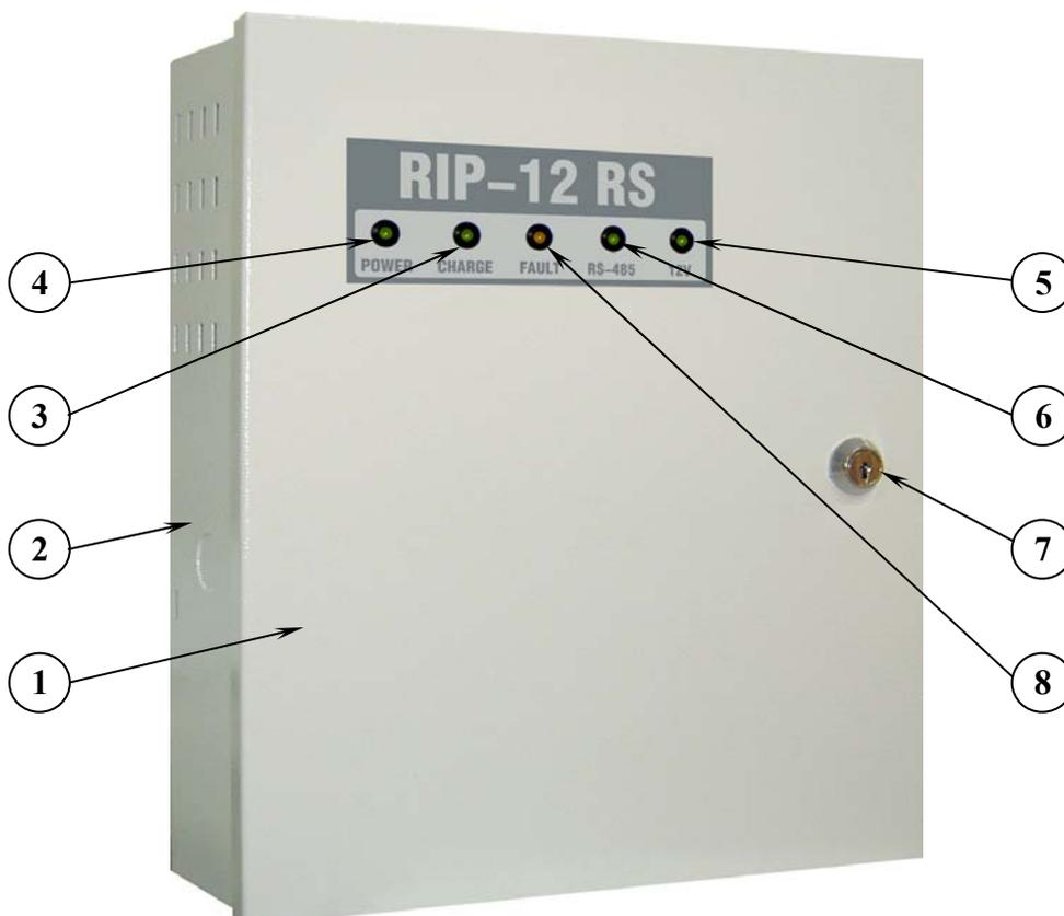
RIP-12 RS is equipped with five LED indicators to provide local condition and trouble indication. POWER Indicator (4), CHARGE Indicator (3) and 12V Indicator (5) are intended to display conditions of input mains power, battery power charger and DC output. FAULT Indicator (8) signalizes all kinds of occurring internal troubles, while RS-485 Indicator (6) indicates communication condition between RIP-12 RS and a network controller via RS-485 interface line.
