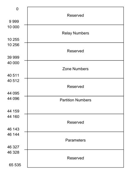
Figure 2. Modbus Registers
