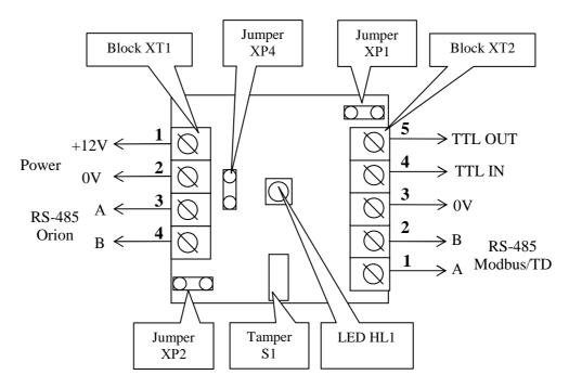
Figure 3. S2000-PP Printed Circuit Board
