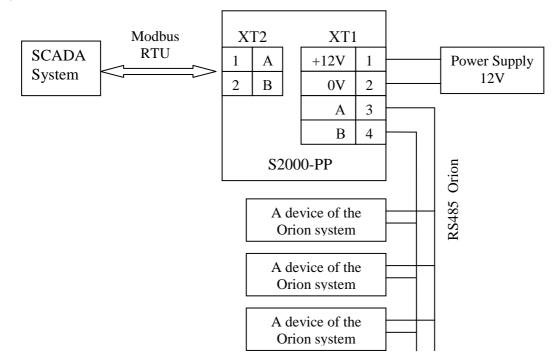
Figure 10. Connecting the S2000-PP in the Orion Master Mode
