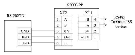
Figure 12. Connecting the Transmitter to the S2000-PP
