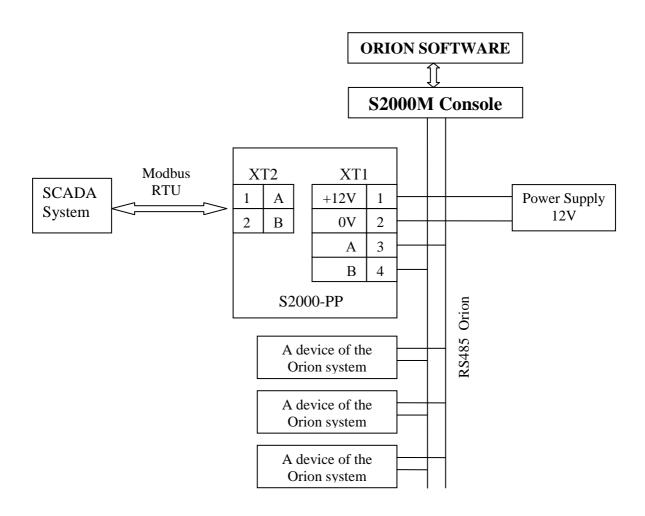
Figure 11. Connecting the S2000-PP in the Orion Slave Mode
