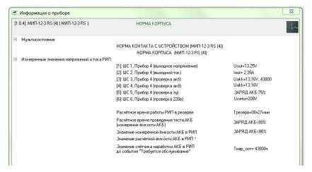
This information window provides access to the ShPS-12 battery measurement control.
